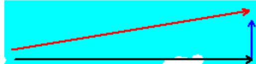
$$10 \text{ m/s [N]} + 60 \text{ m/s [E]} = 60.8 \text{ m/s [E } 9.5^\circ \text{ N]}.$$
